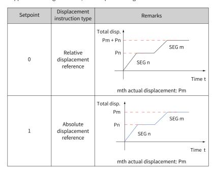
When the actual displacement is a negative value, the motor runs in the reverse direction.
