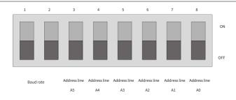
Figure 5-3 DIP switch of H3U
