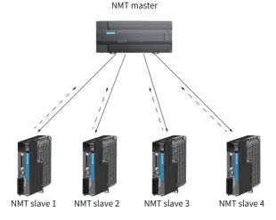
Figure 4-7 Description of node protection
