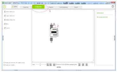
8. The **Add device** dialog box is displayed. Add a CANopen gateway, select **Schneider Electric** for **Supplier**, select **CANopen Optimized**, click the **Add and close**.
