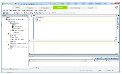
4. Choose **Tools** > **Device Repository** in the toolbar. The **Device Repository** dialog box is displayed. (If the EDS file is imported, steps Step 4 to 6 can be omitted.)
