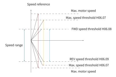
Figure 6-1 Example of speed reference limit
