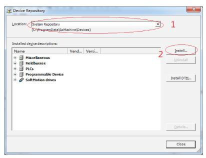
5. As shown in the preceding interface, select **System Repository** and click **Install**. Select a directory for saving the EDS file, as shown below.
