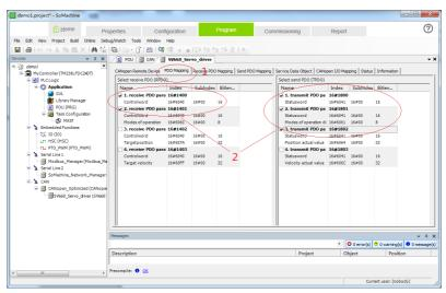
15. Double-click **RPDO1**. The **PDO Properties** dialog box is displayed. Modify **Transmission Type** to **Type 255**. Perform the same operation for other PDOs.
