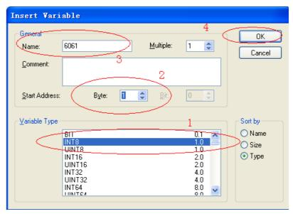
22. You can see that two objects are added to TPDO1. Note that the sequence of the two variables must be the same as that in "Table 5–1 Example of PDO mapping of Beckhoff master" on page 76. Otherwise, the second variable must be deleted and inserted again and a large value must be entered in 2 marked in the figure in Step 21.
