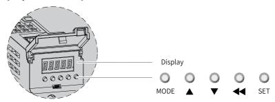
Figure 2-1 Magnified view of the keypad
