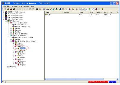
21. For the inserted variable 6061h, select **INT8** (the object dictionary can be queried) for **Variable Type**, enter a large value for **Byte** of **Start Address** to prevent 6061h from being inserted in front of 6041h, enter a proper name, Click **OK**.
