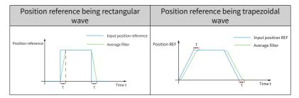
This function does not affect the displacement value (position reference sum). An excessively high setpoint delays the responsiveness, so set a proper filter time constant based on actual conditions.
