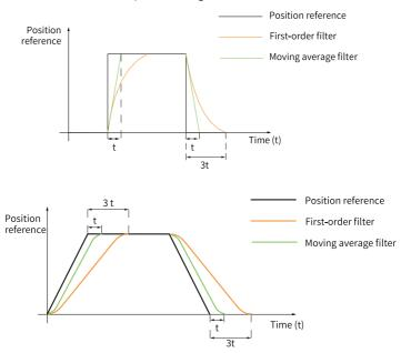
This function does not affect the displacement value (position reference sum). An excessively high setpoint delays the responsiveness, so set a proper filter time constant based on actual conditions.
