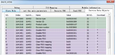
During commissioning, you can monitor the device status online and read/write the object dictionary of the slave through H3U, as shown below.
