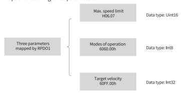
Figure 4-12 Example of PDO1 mapping
