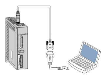
Figure 3-8 Outline drawing of the PC communication cable
