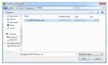
6. Click Open. The EDS file of the SV660C servo drive is imported into SoMachine. In the Device Repository dialog box, you can choose Field Bus > CANopen > Remote Device to view devices..
