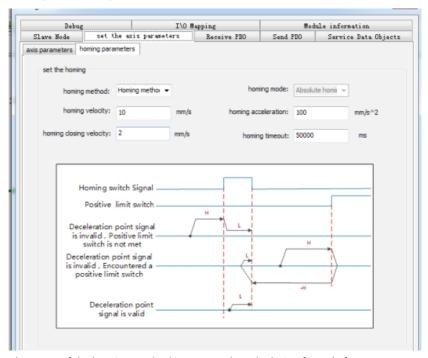
The range of the homing method is 1 to 35. The calculation formula for parameters and object dictionaries of the homing speed, homing acceleration, and homing proximity speed is shown as follows.
