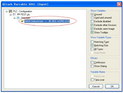
35. After the variable is linked, a small arrow pointing upper right appears at the bottom left of the variable name icon. As shown in the following figure, the name of
