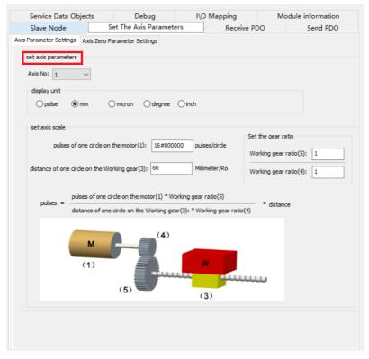
• For devices without reducers, set the gear ratio to 1:1. Set the pulses per motor revolution and distance per motor revolution correctly. The calculation formula is as follows.
