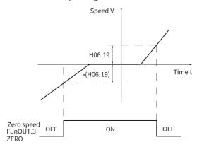
Note: In the preceding figure, "ON" indicates the V-Zero (zero speed) signal is active. "OFF" indicates the V-Zero (zero speed) signal is inactive.
