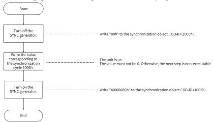
Figure 4-16 Synchronization generator configuration flowchart
