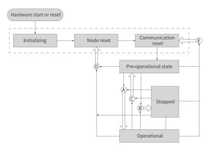
Figure 4-6 Execution process of NMT state machine
