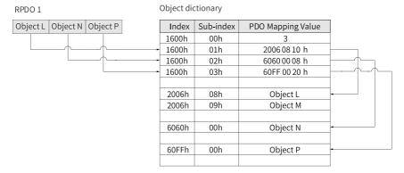
Figure 4-13 Example of RPDO mapping relation
