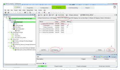
17. Select the proper mapping object in the dialog box displayed according to "Table 5–2" on page 96.
