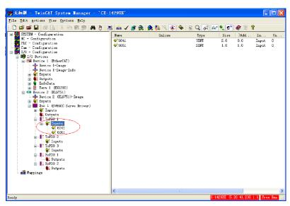
23. Repeat steps 18 to 22 for other PDOs. Add corresponding mapping variables according to "Table 5–1 Example of PDO mapping of Beckhoff master" on page 76. The interface after variables are added is shown below.
