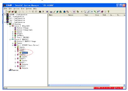
19. Map different variables in each PDO according to "Table 5–1 Example of PDO mapping of Beckhoff master" on page 76. TPDO1 maps 6041h.00hh and 6061h.00hh. To insert the first variable 6041h, select UINT16 in the Variable Type first, and then enter a proper name in the field Name and click OK.
