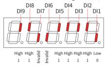
View also the DI terminal logic in group H03 when checking whether a DI function is valid.
