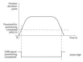
The positioning completed signal is valid only when the servo drive is in running state and in position control.
