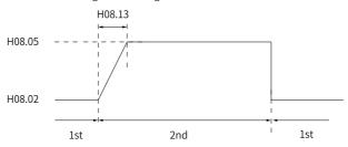
If the set value of H08.05 is no more than that of H08.02, H08-13 will be invalid and the servo drive switches to the 2nd gain immediately.
