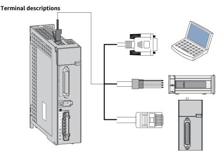
Figure 3-2 Wiring of communication cables
