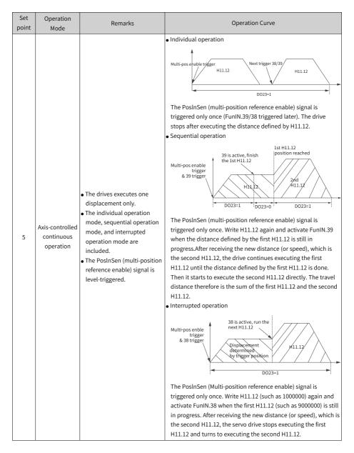
To use the multi-position function, assign FunIN.28 (PosInSen, multi-position reference enable) to a DI first. See "Group H03: Terminal input parameters" for the setting mode.
