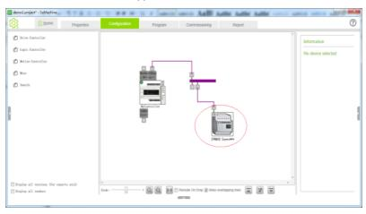
12. Click **Program** and double-click **CAN** on the left to select a proper baud rate. 500 Kbps is selected here.
