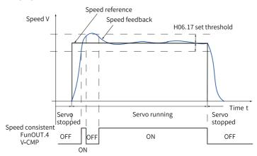
In the preceding figure, "ON" indicates the the V-Cmp (speed matching) signal is active. "OFF" indicates the V-Cmp signal is inactive.
