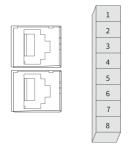
Figure 4-2 Communication Terminal pin layout of the servo drive
