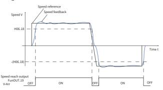
Note: In the preceding figure, "ON" indicates the V-Arr (speed reached) signal is active. "OFF" indicates the V-Arr (speed reached) signal is inactive.
