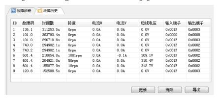
Read the value of H0b.34 to get the fault/warning code. See examples in the following table.
