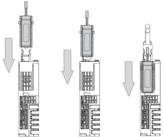
Figure 3-30 Installing the battery box (bottom view)
