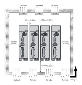
Figure 1-4 Clearance for compact installation
