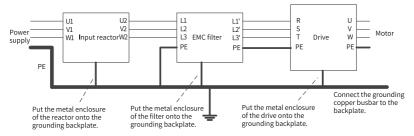
Figure 1-12 Installing the AC input reactor
