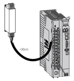
Figure 3-16 Installing the filter
