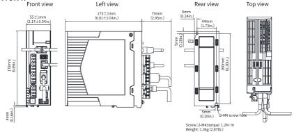
Figure 1-8 Dimension drawing of servo drives in size C
