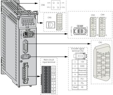
Figure 3-1 Terminal pin layout of servo drives in size A
