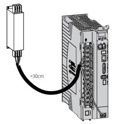
Figure 1-13 Installing the AC input reactor
