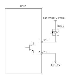
When the host controller provides relay input, a flywheeling diode must be installed. Otherwise, the DO may be damaged.
