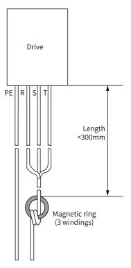
Figure 6-1 Magnetic ring on the input side
