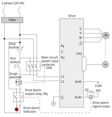
Figure 3-17 Main circuit wiring
