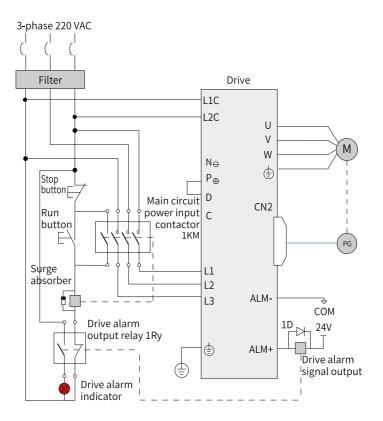
Figure 3-18 Main circuit wiring of three-phase 220 V models
