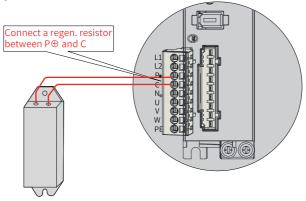
Figure 3-39 Wiring of external regenerative resistor
