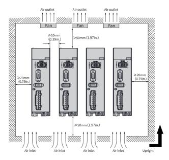
Figure 1-3 Clearance for side-by-side installation
