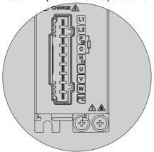
Figure 3-8 Main circuit terminal pins of size A drive
