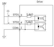
Wiring example for an internal 24 V
