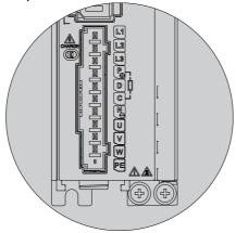
Figure 3-9 Pin assignment of main circuit terminal of servo drives in size B
