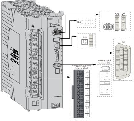
Figure 3-5 Terminal pin layout of servo drives in size E
