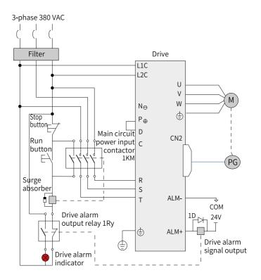
Figure 3-19 Main circuit wiring of three-phase 380 V models
