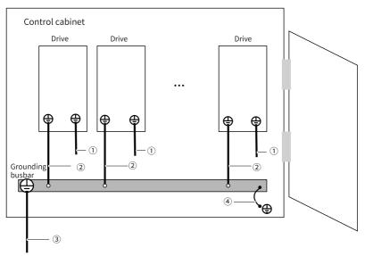
Table 3-21 Description for grounding of multiple drives installed side by side
