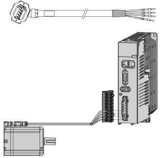
Figure 3-14 Wiring between the servo drive and terminal-type motor
