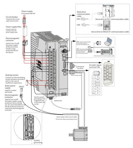
Figure 2-3 Wiring example of a three-phase 380 V system
