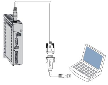
Figure 3-38 Serial-to-USB conversion
