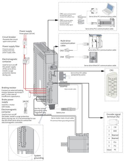
Figure 2-1 Wiring example of a single-phase 220 V system
