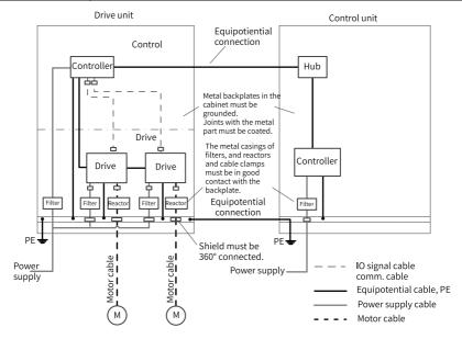
Figure 3-20 Recommended wiring for the control cabinet system
