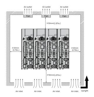
Figure 1-5 Zero-clearance installation
