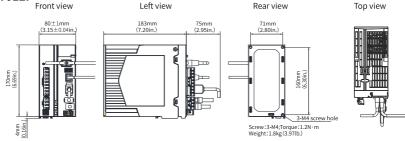
Figure 1-9 Dimension drawing of servo drives in size D
