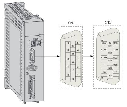
Figure 3-22 Control terminal pin layout of servo drives in sizes A and B
