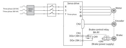
Figure 3-25 Wiring of the brake
