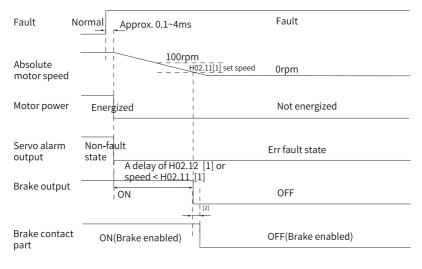
Figure 2-11 Sequence of "Dynamic braking stop, keeping dynamic braking status" at No.
