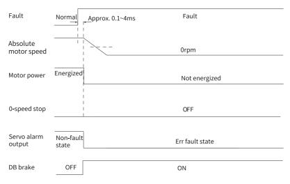
Figure 2-12 Sequence diagram of "Dynamic braking stop, keeping dynamic braking sta-
