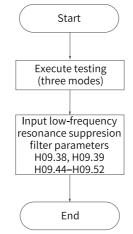
Figure 3-16 Procedure for setting low-frequency resonance suppression filter
