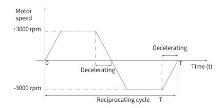
Figure 2-5 Example of motor speed curve (without external load torque)
