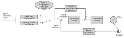
Figure 3-10 Block diagram of torque feedforward control
