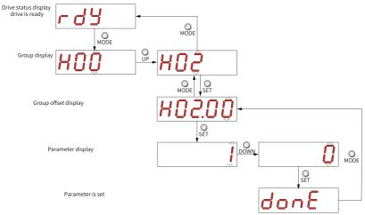
Figure 1-6 Example of parameter setting
