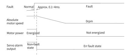
Figure 2-9 Sequence of "Coast to stop, keeping de-energized state" at No. 1 fault
