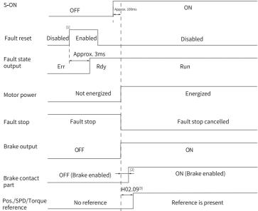
Figure 2-18 Sequence for fault reset
