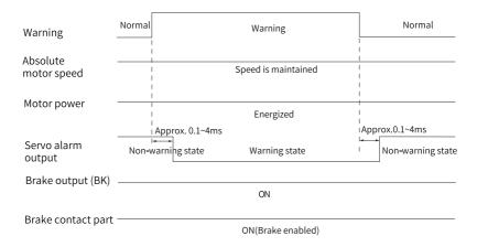
Figure 2-17 Sequence for warnings that do not cause stop
