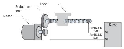
Figure 2-19 Installation of limit switches
