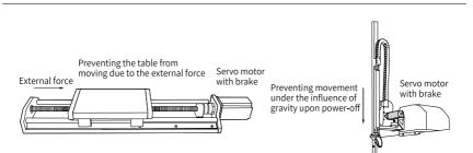
Figure 2-2 Application of the brake
