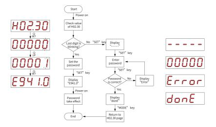
Figure 1-16 Procedure for setting the user password
