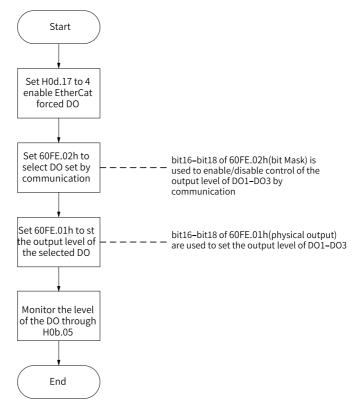
Figure 1-14 Procedure for setting EtherCAT forced DO
