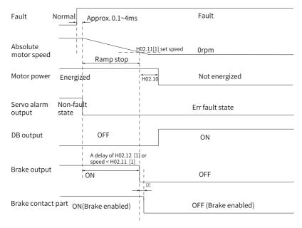
Figure 2-15 Sequence of "Ramp to stop, keeping dynamic braking status" at No. 2 fault
