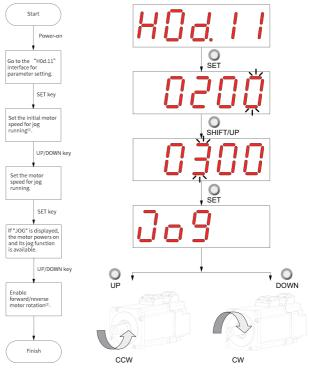
Figure 2-1 Procedure for setting the jog function
