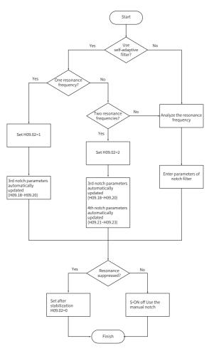
Figure 3-13 Using the notch
