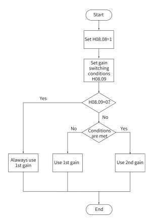
Figure 3-8 Gain switchover flowchart when H08.08 is set to 1
