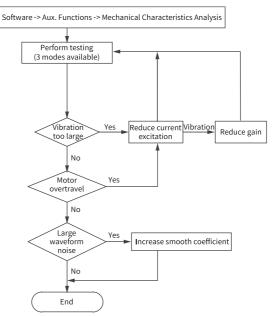
Figure 3-18 Operating procedure for mechanical characteristic analysis
