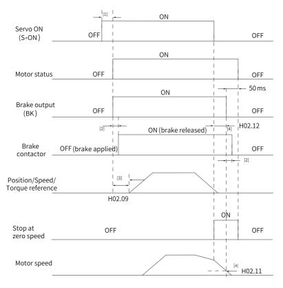
Figure 2-4 Brake sequence for a rotating motor
