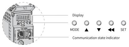
Figure 1-1 Magnified view of the keypad
