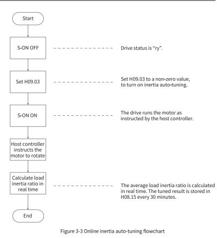
H09.03 defines the real-time updating speed of the load moment of inertia ratio (H08.15).
