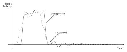
Figure 3-17 Low-frequency resonance suppression effect
