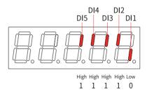
Figure 1-9 DI level status corresponding to H0b.03
