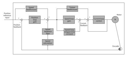
Figure 3-6 Basic control for manual gain tuning
