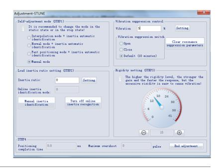
To ensure a stable operation of STune mode 4 with default parameter settings, gain parameters will be adjusted along with the inertia ratio when the inertia ratio is higher than 13. In multi-axis trajectories, responses may be inconsistent under the same stiffness level.
