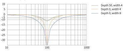
The following figure shows the frequency characteristics of the notch.
