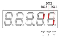
Figure 1-15 Display of H0b.05 when DO signals are controlled by EtherCAT
