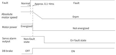
Figure 2-13 Sequence of "Dynamic braking stop, keeping dynamic braking state" at No.
