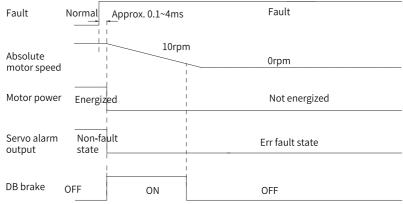
Figure 2-10 Sequence of "Dynamic braking stop, keeping de-energized state" at No. 1
