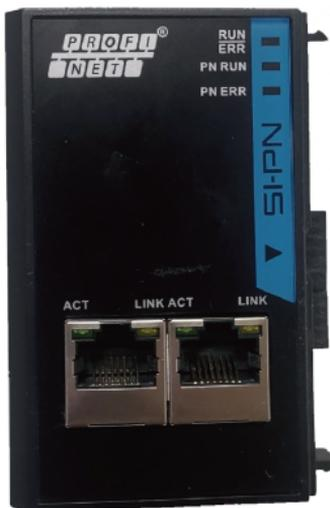
Figure 1-1 SI-PN communication expansion card appearance
