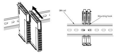
**Note:** After the module is installed, the DIN rail mounting hook will automatically move downward to lock the module to the rail. If the hook does not move downward, press down the top of the hook to ensure that the module is installed in place.
